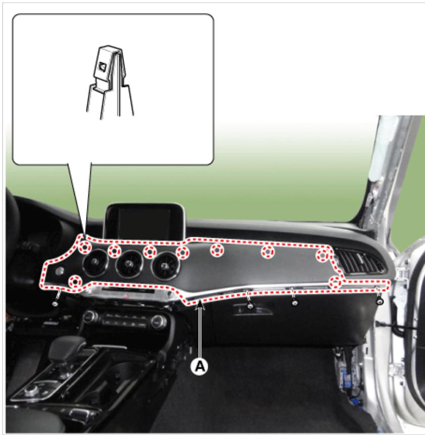
4. Disconnect the start/stop button connector (A) and then remove the crash pad garnish.
