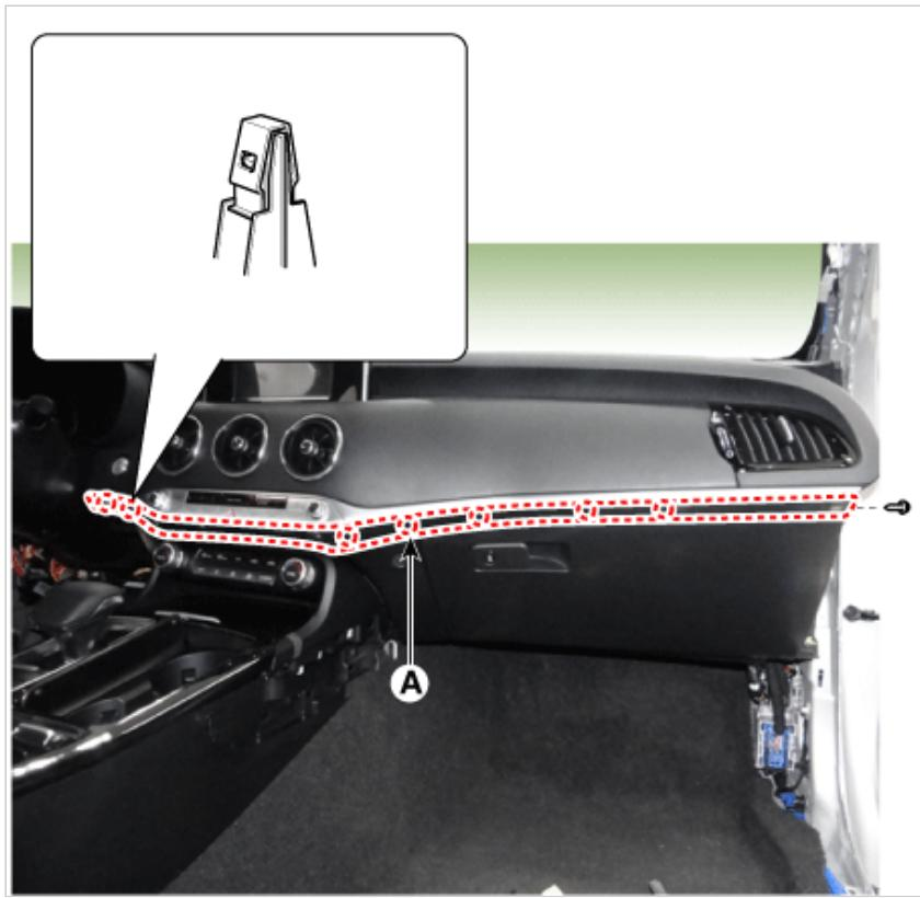
3. Separate the crash pad passenger side panel (A) after loosening the mounting screws.
