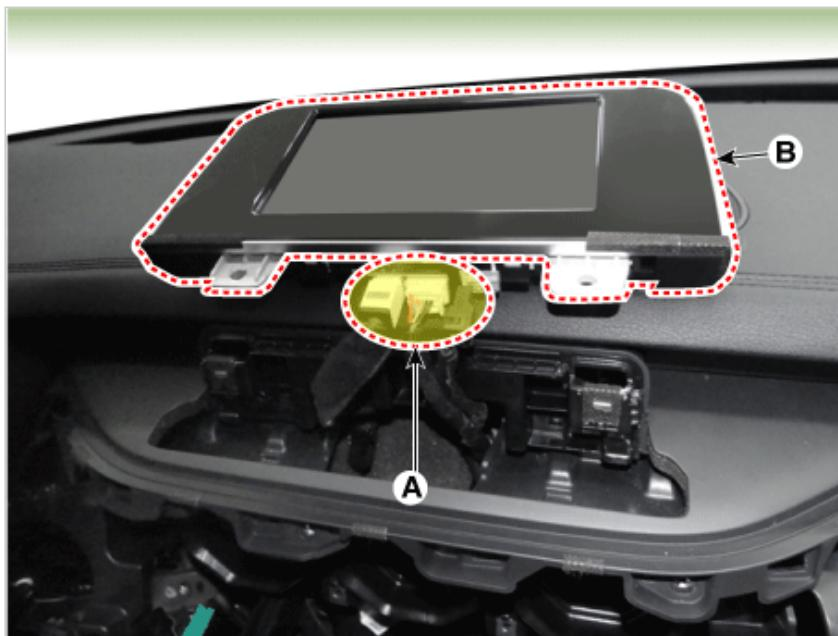
7. Remove the monitor fascia panel (A) after loosening the mounting screws.
