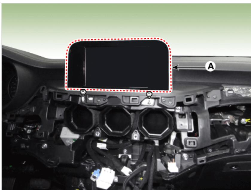
6. Remove the monitor assembly (A) after disconnecting the connectors.
