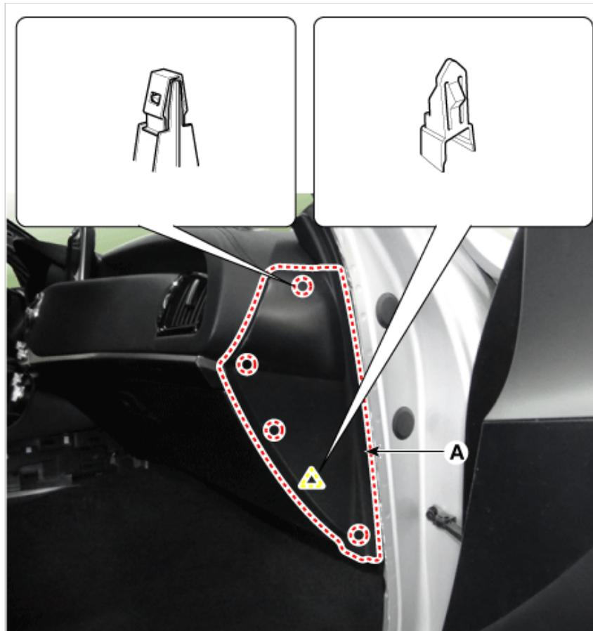
2. Remove the crash pad garnish [RH] (A) after loosening the mounting screws.
